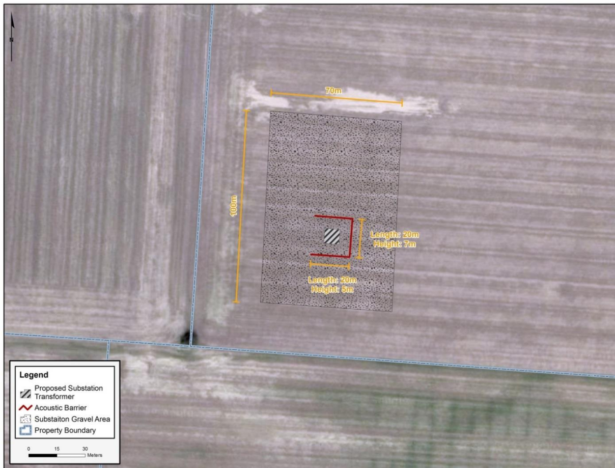
Figure 4-1 Romney acoustic barrier and gravel area dimensions
