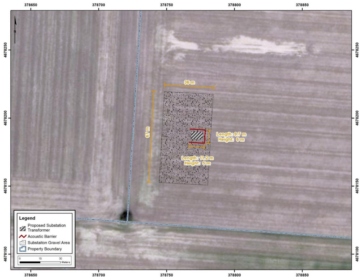
Figure 4-1 Romney acoustic barrier and gravel area dimensions
