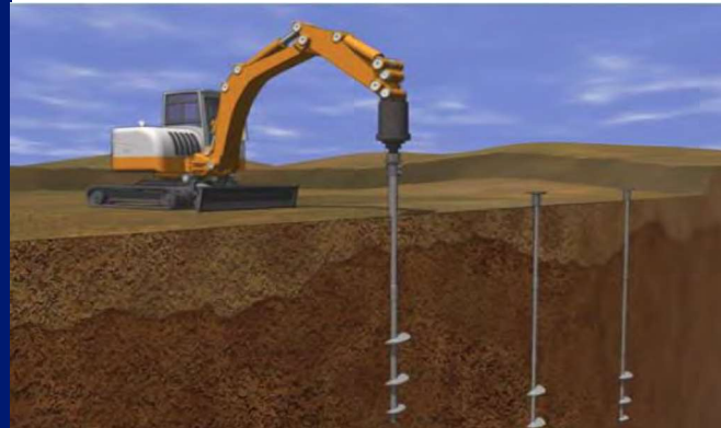
Helical Pile Installation (usually about 8' deep)
