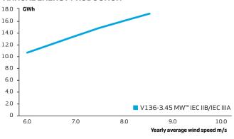
One wind turbine, 100% availability, 0% losses, k factor =2, Standard air density = 1.225, wind speed at hub height
