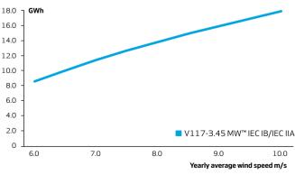
Assumptions One wind turbine, 100% availability, 0% losses, k factor =2, Standard air density = 1.225, wind speed at hub height
