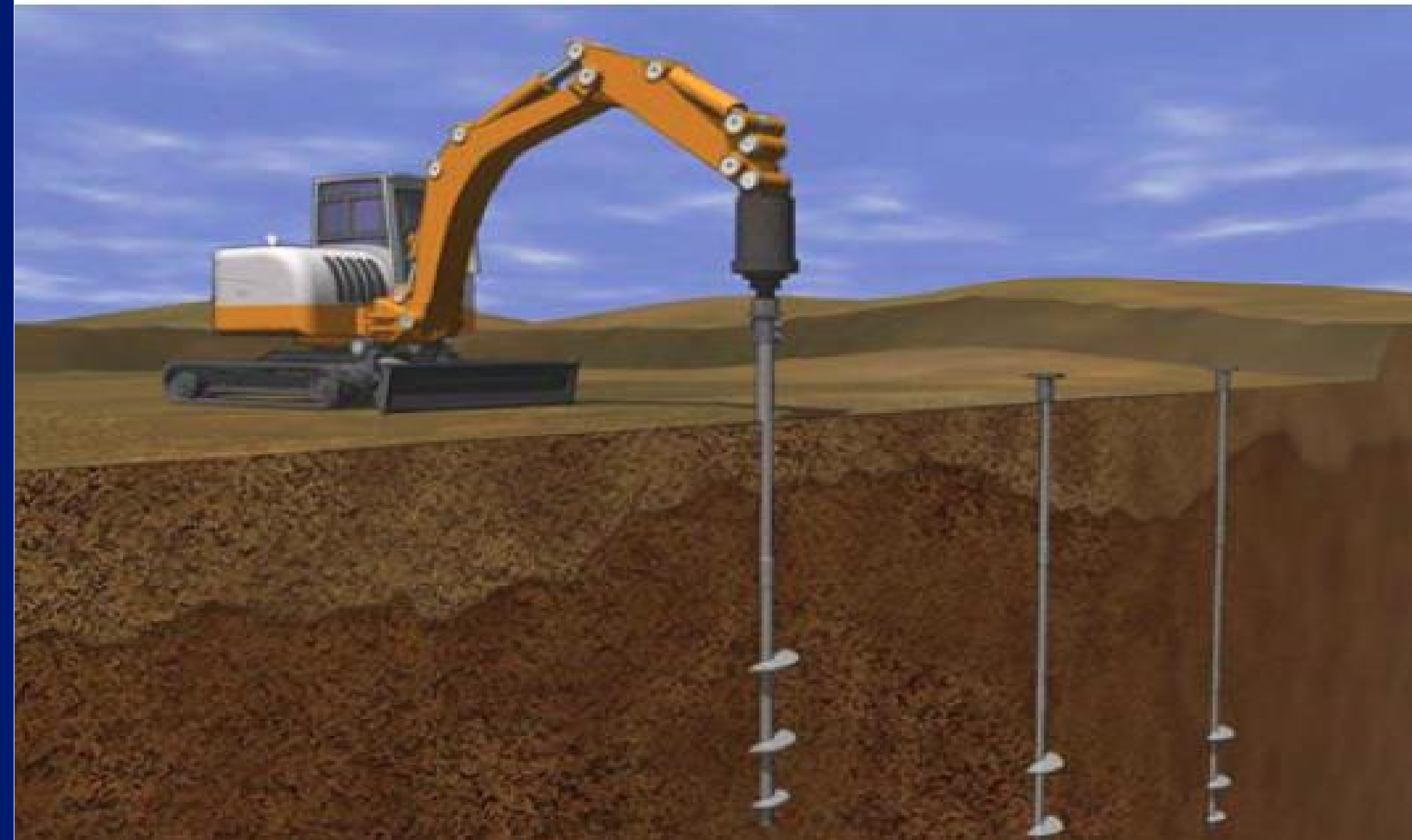
Helical Pile Installation (usually about 10' deep)
